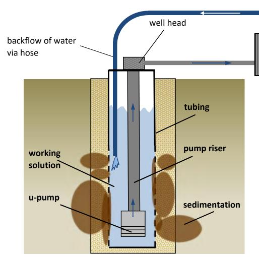
To set up the circulation flushing a branch with a hose connection (T-piece) must be installed after the heat pump.
